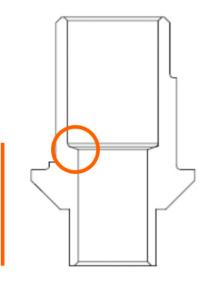
The 19° seating design has a distance from the seating of the screw to the implant which is longer than the BioHorizons<sup>®</sup> compatible tibase and the hex is 2.425mm.
